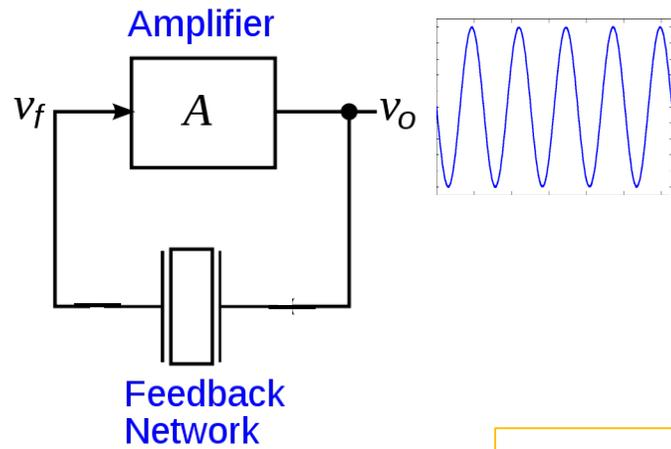
An electronic oscillator circuit that uses the mechanical resonance of a vibrating crystal of piezoelectric material to create an electrical signal with a very precise frequency.
